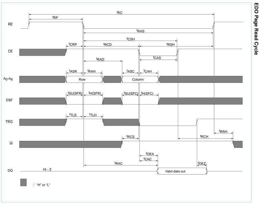
IBM025170 IBM025160 IBM025171 IBM025161 **256K X 16 MULTIPORT VIDEO RAM**
