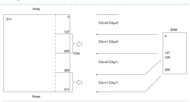
The example illustrates a full transfer in SRS mode based on CA<sub>7</sub>=1.
